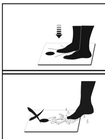
AUTO STEP ON – just step on the scale and stand still, the scale will automatically turn ON and start taking measurements.
