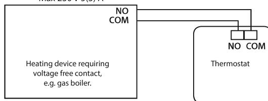
\* In case of NC boiler, the thermostat should be set to COOLING mode.
