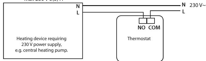
\* In case of NC boiler, the thermostat should be set to COOLING mode.
