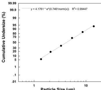
Measurements were performed using a sodium fluoride solution with a "Next Generation Impactor" (NGI). The diagram may therefore not be applicable to suspensions or highly viscous medications. You can obtain more detailed information from the manufacturer of your medication.
