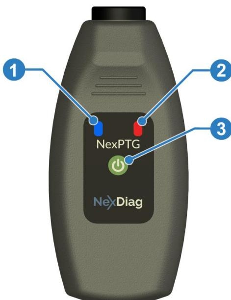
In order to start the **NexPTG** gauge the button ③ should be held down for three seconds until the power diode lights up on the panel ②. Next, start the **NexPTG** application on the mobile device (external). Correct communication will be signaled by the lighting up of the blue diode ①.
