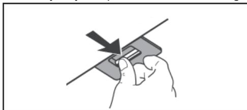
The activated charcoal filter is not washable and cannot be regenerated, and must be replaced approximately every 4 months of operation, or more frequently for particularly heavy usage.
