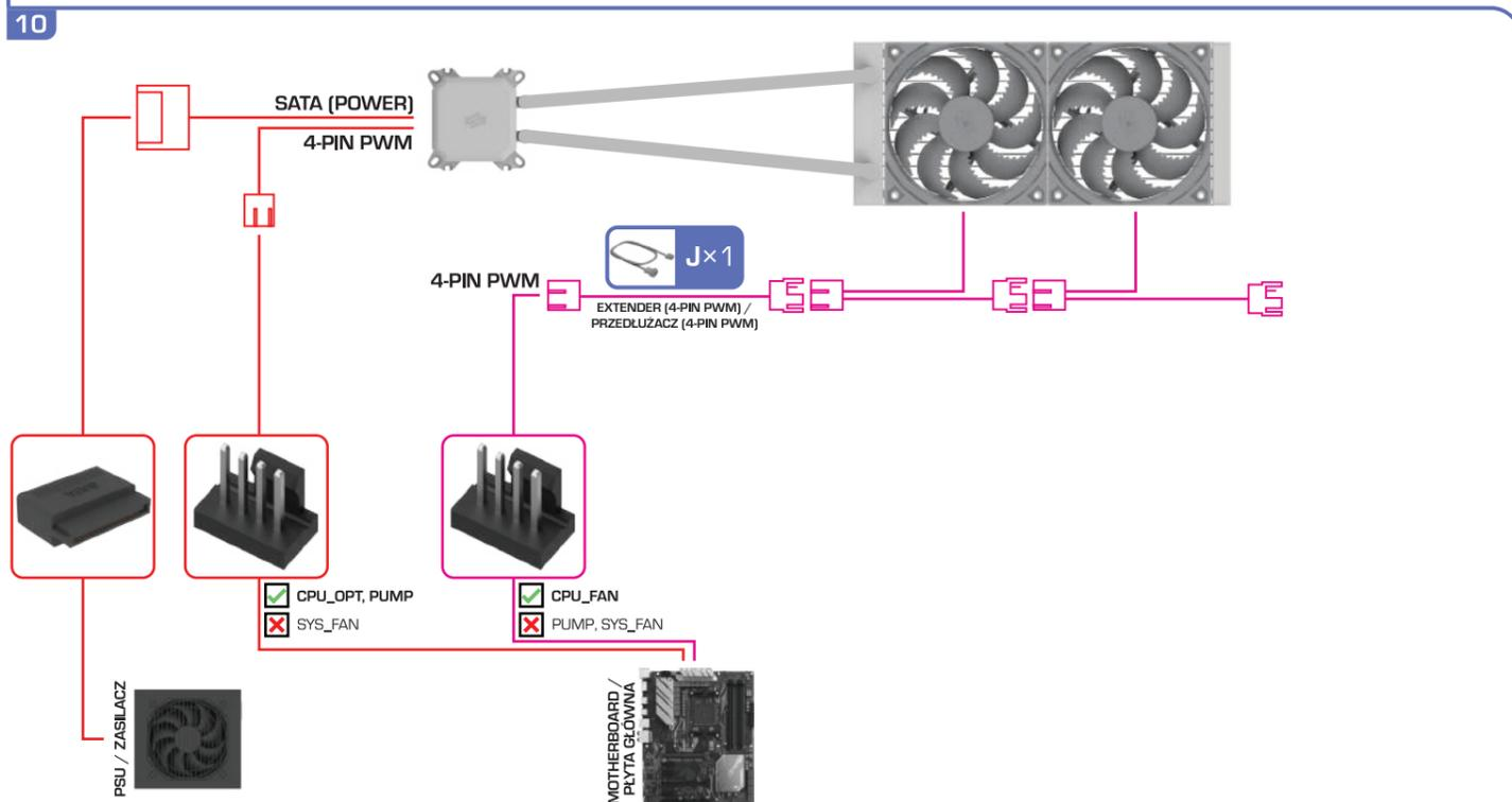
EN: The red line shows how to correctly connect the pump. Connect the power to a SATA plug and control signal to a 4-pin fan connector. Configure your motherboard for speed control in PWM mode (consult the motherboard manual for details).
