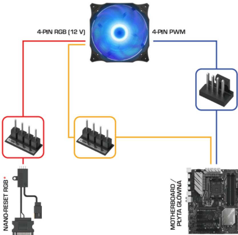
**A** EN: Choose A if you have a motherboard with 4-pin RGB socket and want to control the ARGB lighting using the software from your motherboard manufacturer. If you chose B (control via motherboard), connect the individual elements according to the yellow lines only.
