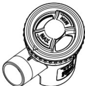
To make the inhalation therapy faster, turn the speed selector (C1.2.3) clockwise.
