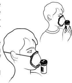
6. Start the device by means of switch (A1) and breathe deeply in and out. After inhaling, we recommend holding your breath for an instant to allow the inhaled drops of aerosol to deposit. Then exhale slowly.
