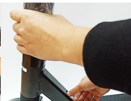
folding Strengthen outwards the column and press the button by other hand same time
