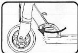
3. Open the locking mechanism.
