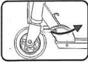
4. Lock the locking mechanism.
