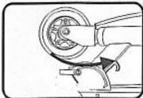
1. Unlock the locking mechanism.
