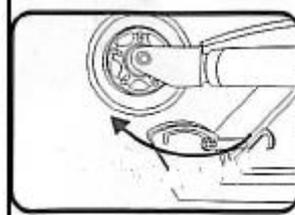
6. Lock the locking mechanism.
