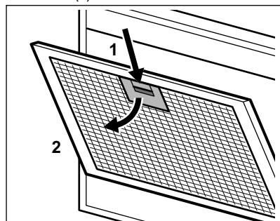
3. Slightly tilt the front of the filter downwards (2), then pull. Repeat the first two steps for all filters.
