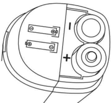
3. Place the cover back onto the battery compartment until you feel it click into place.
