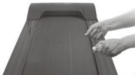
Pull up tightly of the running belt. Then put the silicone oil to running board. Then start the machine to running 3 minutes without loading. It is better to maintain like this every 30 hours working of the machine. This can save lifetime of parts properly.
