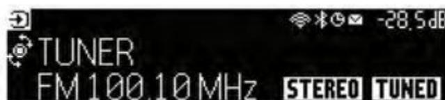
"TUNED" lights up on the front display when the unit is receiving a radio station signal.
