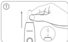
Remove the output shaft sleeve in correct direction.
