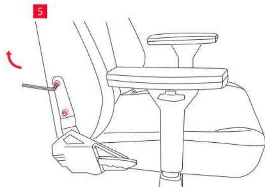
Remove the foam covers from the seat supports, Then carefully position the backrest between the supports. Reinstall the 4 bolts and washers on the sides of the backrest. Tighten all the bolts at the same time until they fit precisely.
