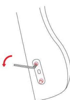
Remove the factory-fitted bolts and washers from the backrest, use the hex wrench.
