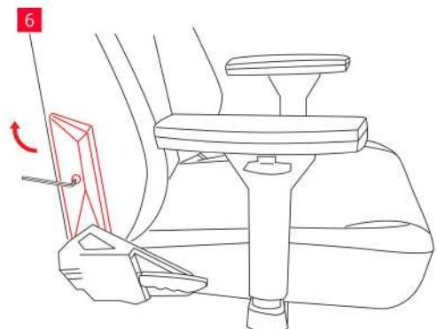
Install the side covers, and then tighten the screws. The cover marked with the letter "R" must be installed on the side of the lever for angle adjustment of the backrest.
