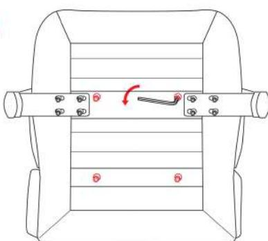
Place the chair on the backrest. Remove the 4 screws and washers from the bottom of the seat.
