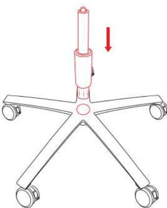
Insert the gas lift into the base by pushing.
