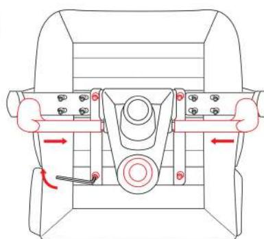
Align the mechanism with the holes on the underside of the seat, the "FRONT" arrow must be pointing towards the front of the seat. Reinstall the washers and bolts, and then tighten them evenly.
