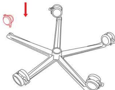
Insert each wheel into the base by pushing.
