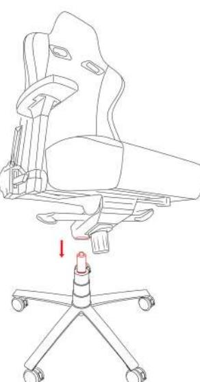
Install the top of the chair on the gas lift.
