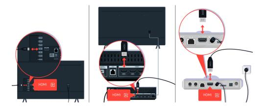
Check the antenna and HDMI cable connections.
