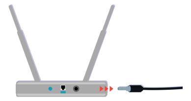
Try rebooting the access point by disconnecting and reconnecting the power connector. It may take 1 to 2 minutes until the access point comes back online after a reboot.
