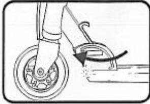
3. Open the locking mechanism.
