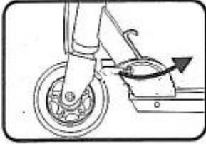
4. Lock the locking mechanism.
