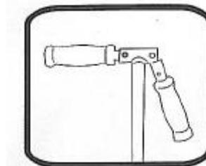
2. Remove both handles from the transverse steering wheel tube.
