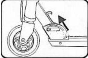
4. Pull the lever upwards.
