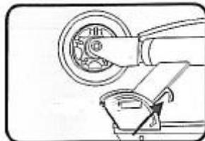
2. Pull the lever upwards.
