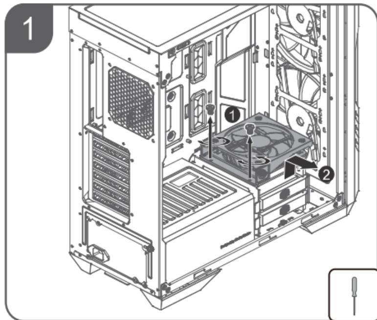
\*(Fan and fan mount needs to be removed completely)
