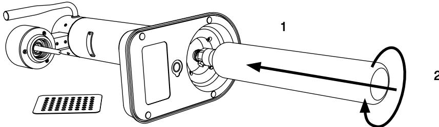
Unscrew the plastic seal from the top of the gas cylinder, and carefully insert it into the Aarke Carbonator through the hole at the bottom. Don't drop the cylinder into the hole. When you feel it reach the top, begin to screw the cylinder in with a clockwise motion until fastened. Be careful not to screw it in too hard, as this could rupture the threads holding the cylinder in place.
