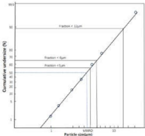
Measurements were performed using a salbutamol solution with a “Next Generation Impactor” (NGI).
