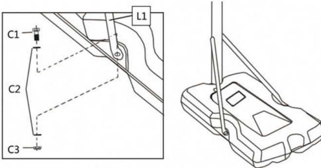
Fix the other end of Pole Brace (L1) & (L2) on two sides of Base (S) by Bolt Set (C1), (C2) & (C3) as shown.
