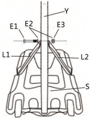
Fix one end of Pole Brace (L1) & (L2) on Bottom Pole (Y) by Bolt Set (E1), (E2) & (E3) as shown.
