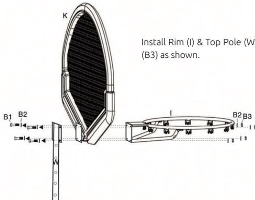
Install Rim (I) & Top Pole (W) on Backboard (K) by Bolt Set (B1), (B2) & (B3) as shown.
