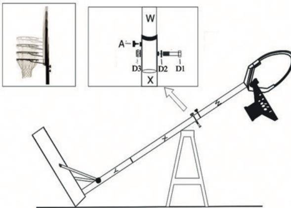
Insert the Top Pole (W) into Middle Pole (X), adjust it to required height, then fix them by Plastic Head Knob (A) & Bolt Set (D1), (D2) & (D3) as shown. Adjust the height by change the Bolt Set (D1), (D2) & (D3) in different holes on Top Pole (W).
