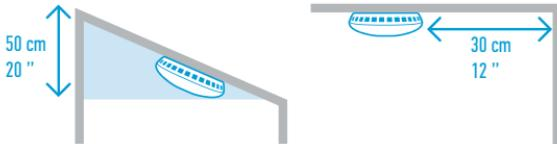
**EN** You are advised to fLV the LTtector on the ceiling. Ensure that the chosen location is at least 30 cm PLoM the wall. In case of a sloping ceiling, fLV the LTtector no more than 50 cm below the highCZt point.
