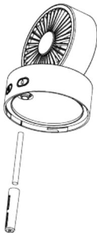
The unit is equipped with a water filter. The water filter requires periodic replacement (depending on the degree of water contamination).
