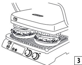
The grease from the food is drained and collected by the grooves on the plate and the hole at the back and is collected in the grease tray.
