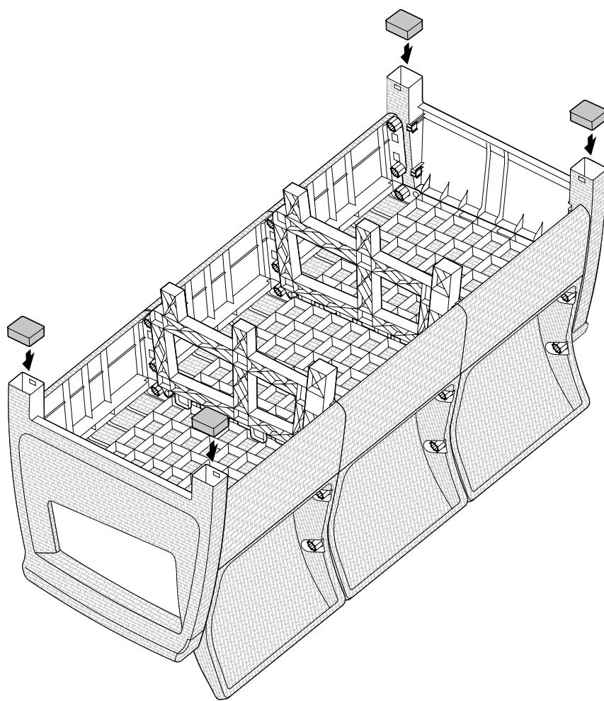
**EN** At this stage, the product is completely assembled. All of the screws should be given a final tightening with a wrench.
