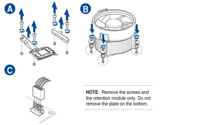
**NOTE:** Remove the screws and the retention module only. Do not remove the plate on the bottom.
