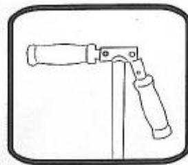
2. Remove both handles from the transverse steering wheel tube.
