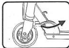
4. Lock the locking mechanism.
