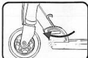
3. Open the locking mechanism.
