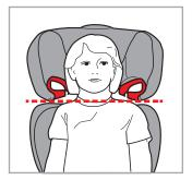
Check to make sure it is clicked into one of the six height positions by pulling up on head support.
