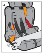
2 Fitting the Child Restraint with the 3-Point Lap & Diagonal Seat Belt
