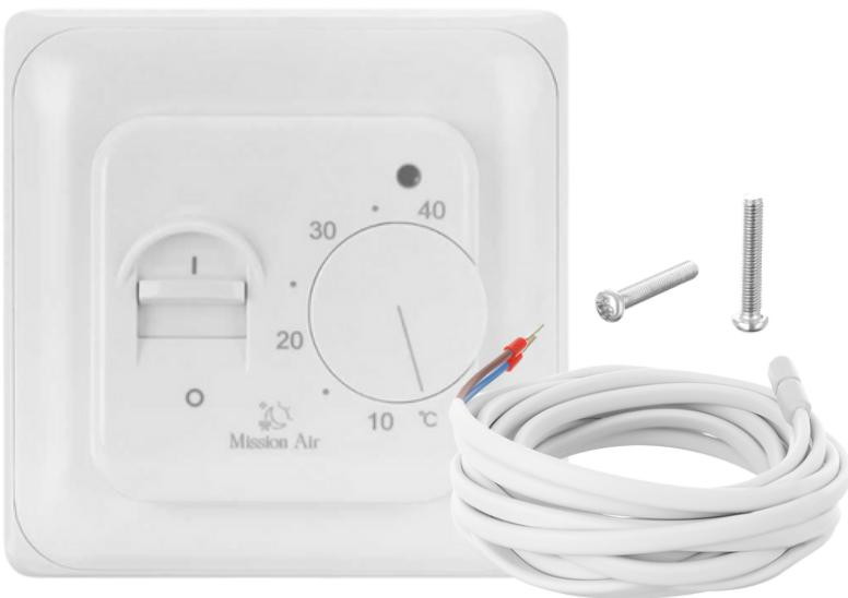
The Mission Air® Aries manual room thermostat is designed to control electric underfloor heating systems. Mounted in a standard 60mm electrical box, the controller operates based on the readings of a wired floor temperature sensor. LED indicates system operation, possible temperature control from 5-40°C.
