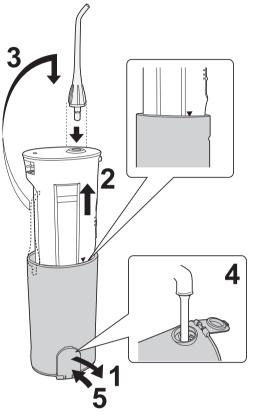
Insert the nozzle into the nozzle socket holding onto the white part of the main unit.
