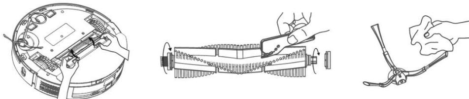
Remove the central cleaning brush by pressing the two tabs on the brush cover. Use the cleaning tool to remove any hair tangled in the main brush. Keep the center cleaning brush free of large amounts of hair, dust, cotton, etc. Check the side cleaning brush together with the air intake opening according to the intensity of the dirt, at least once a week, and remove tangled hair and other dirt.
