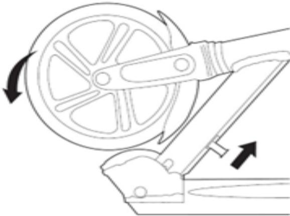
3. To release the folding mechanism, hold the T-tube with one hand between the collar clamp and the quick-release lever and place your foot on the deck plate. With the other hand, pull the joint lever up to release the steering column from the locked position and allow you to pivot it to the upright position.
