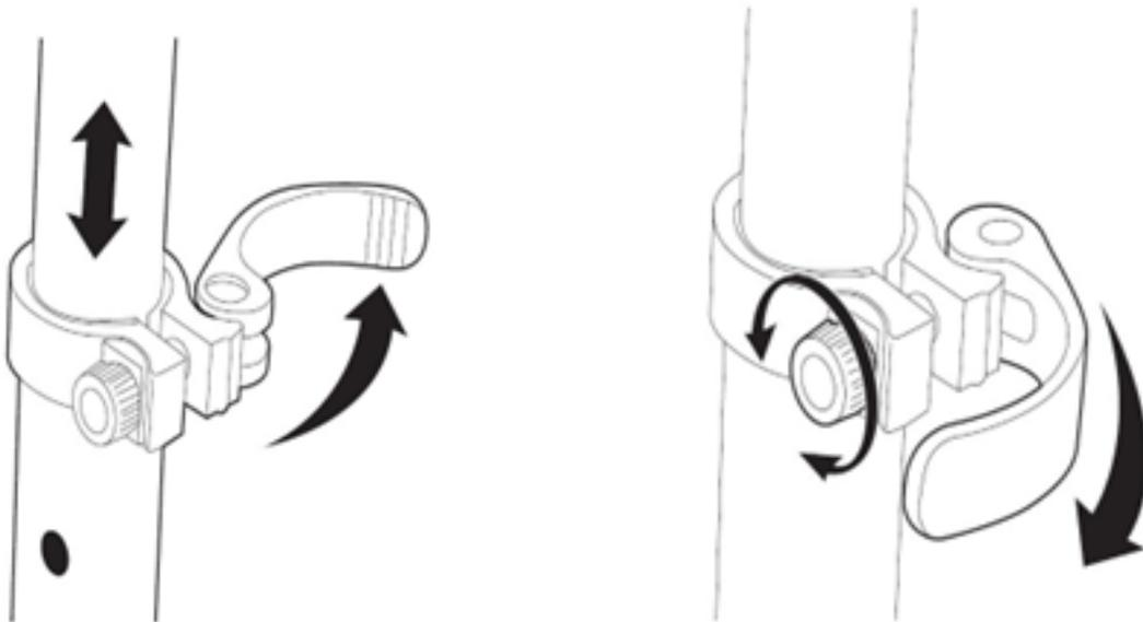
5 To adjust the height of the handlebars, unlock the extension tube by pulling outward on the quick-release lever and pushing the button located on the extension tube. Slide the T-tube to the desired position and secure by pushing inward on the quick release lever
