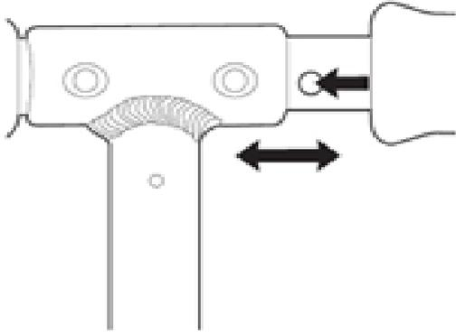
1. Insert and secure the left and right handlebars by pressing the spring-loaded buttons and inserting them into the T-tube.
