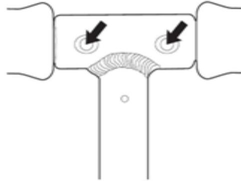
2. Make certain the spring-loaded button engages the hole in the T-bar for each handlebar.
