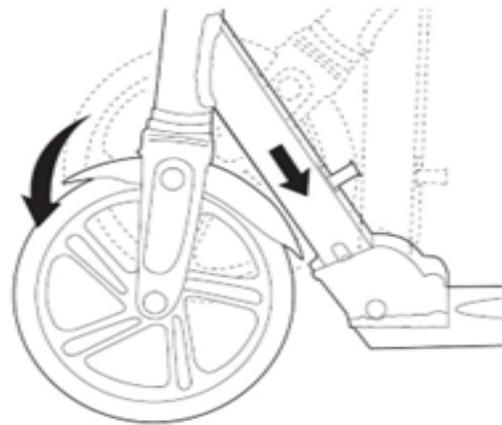
4 The Joint lever is spring-loaded and will automatically lock in the upright position when fully upright.
