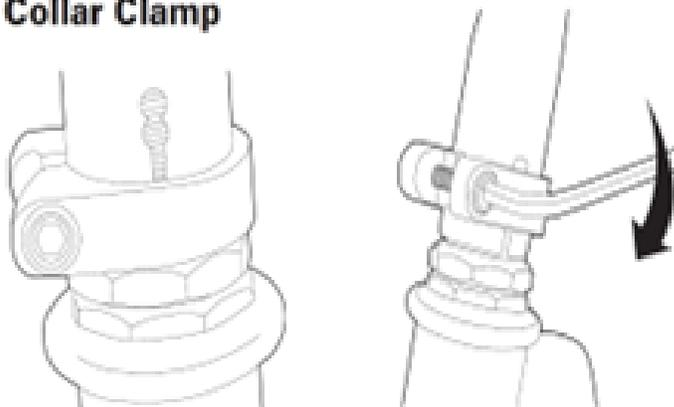
Using the 5mm Allen wrench, check that the collar clamp bolt is tightened securely. This item is tightened and quality inspected at the factory, but there is a slight chance that the effects of shipping or handling may have caused this bolt to loosen.
