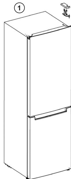
2. Take down the fridge door, pul it aside carefully; then remove the two screws which fix the middle hinge, take down the middle hinge, pul it aside carefully; take down the freezer door, pul it aside carefully.
