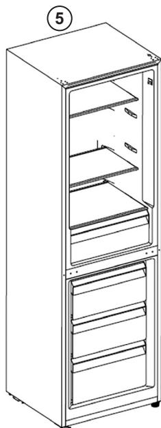
5. Take the freezer door, make sure the down hinge axis and the axis hole on the lower left side on the machine fix well and connect correctly. The freezer door is basically fixed now; then use the two screws to fix the middle hinge on the left side of the cabinet; then fix tight the middle hinge (as shown in the diagram No.6).
