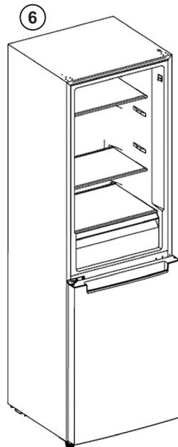
6. Take the fridge door, make sure the down hinge axis and the axis hole on the lower left side on the machine fix well and connect correctly; the fridge door is basically fixed now. Then use the screws which were taken down in the step one, to fix the upper hinge on the left side of the cabinet; then put on the upper hinge cover, then fix it by the screws.
