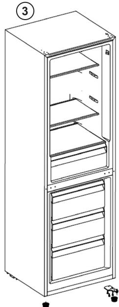
4. Screw the adjustable foot which is on the left side previously to corresponding position of the right side under the cabinet. Turn the down hinge at 180 degrees and fix the down hinge axis on the down hinge axis on the hole of the down hinge. Then twist the hinges and screws tightly; do the same to the adjustable foot which is on the right side previously to corresponding position of the left side under the cabinet; then twist the three screws which fix the down hinge tightly.
