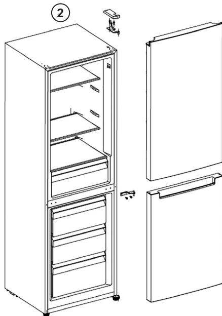
3. Remove the three screws which fix the down hinge under the right side of cabinet. Take down the down hinge and the adjustable foot below the down hinge under the right side of cabinet. At the same time, use spanner to remove the screws which fix the hinge axis, take down the down hinge axis; then remove the adjustable foot on the lower left side under the left side of cabinet.
