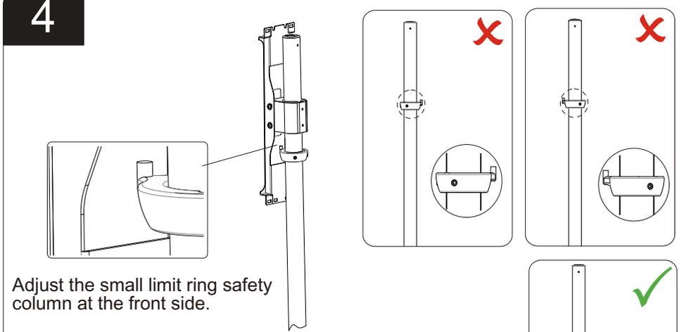
Adjust the small limit ring safety column at the front side.
