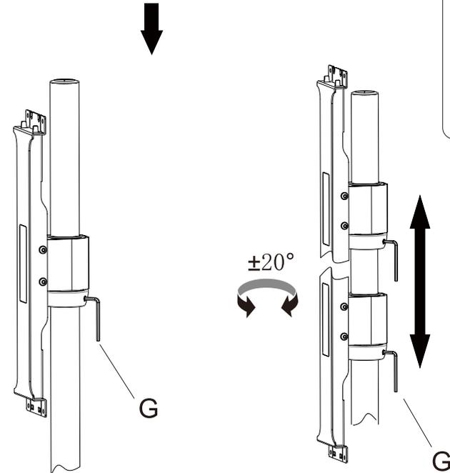
Make the TV panel full assembled into that small limit ring safety colume, lock it on a proper height via G wrench.
