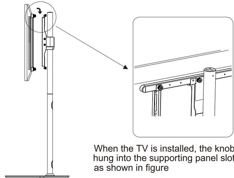
When the TV is installed, the knob is hung into the supporting panel slot as shown in figure
