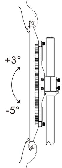
Use G wrench to adjust the screw as shown in figure to achieve the TV up and down flip  $+3^{\circ}$ ~ $-5^{\circ}$
