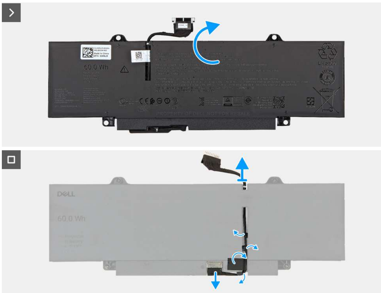
Rysunek 21. Removing the battery and disconnecting the battery cable
