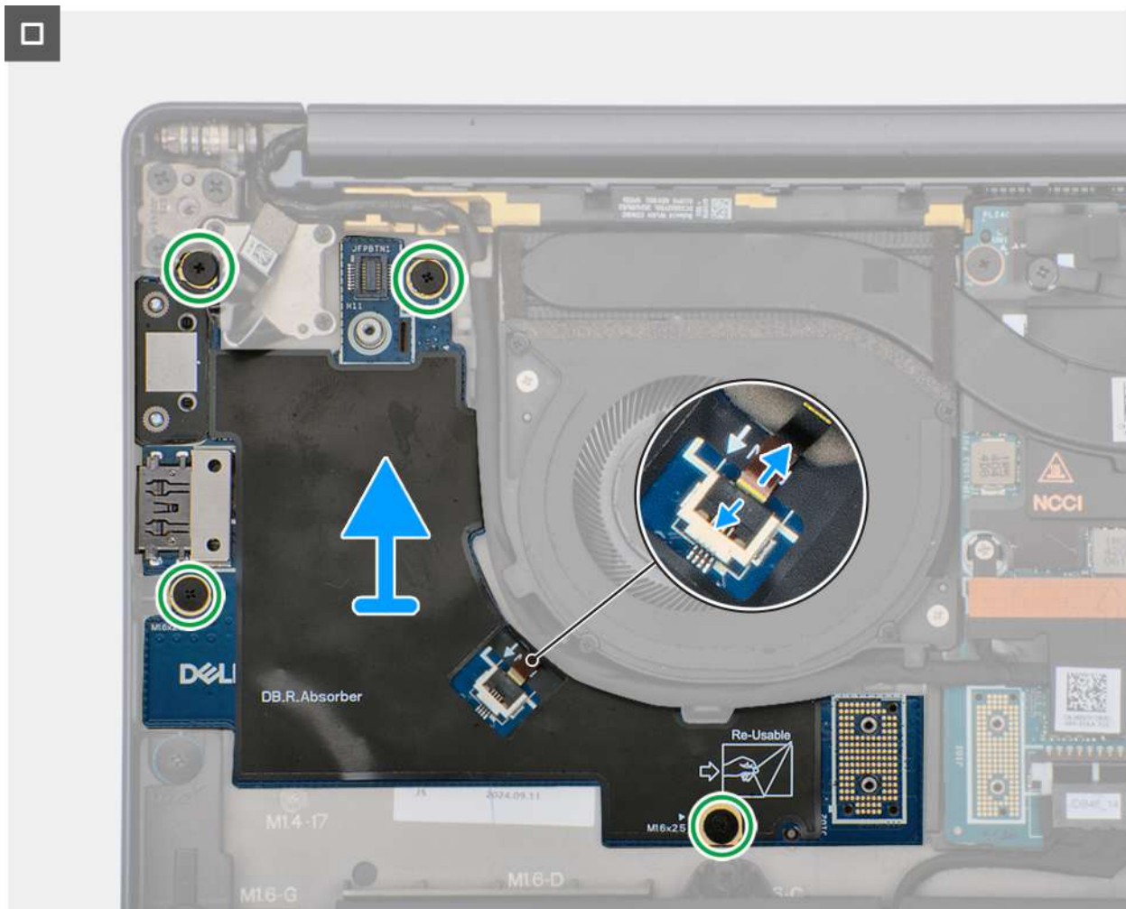
Rysunek 42. Removing the right I/O-board (without WWAN antennas)
