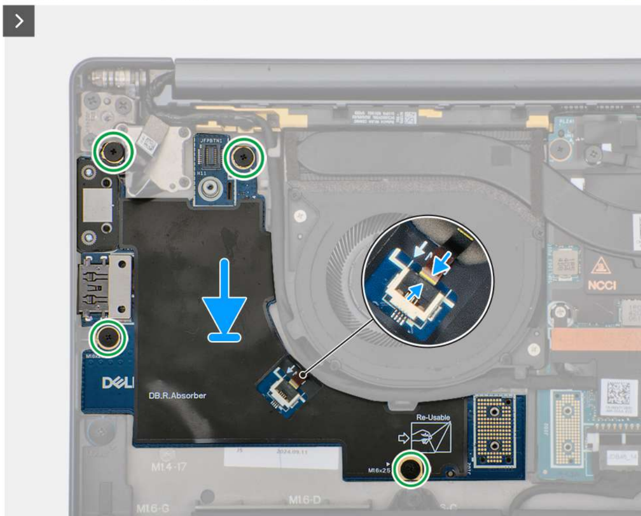
Rysunek 45. Installing the right I/O-board (without WWAN antennas)
