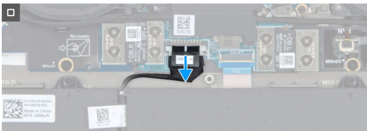
Rysunek 16. Disconnect the battery cable from the system board
