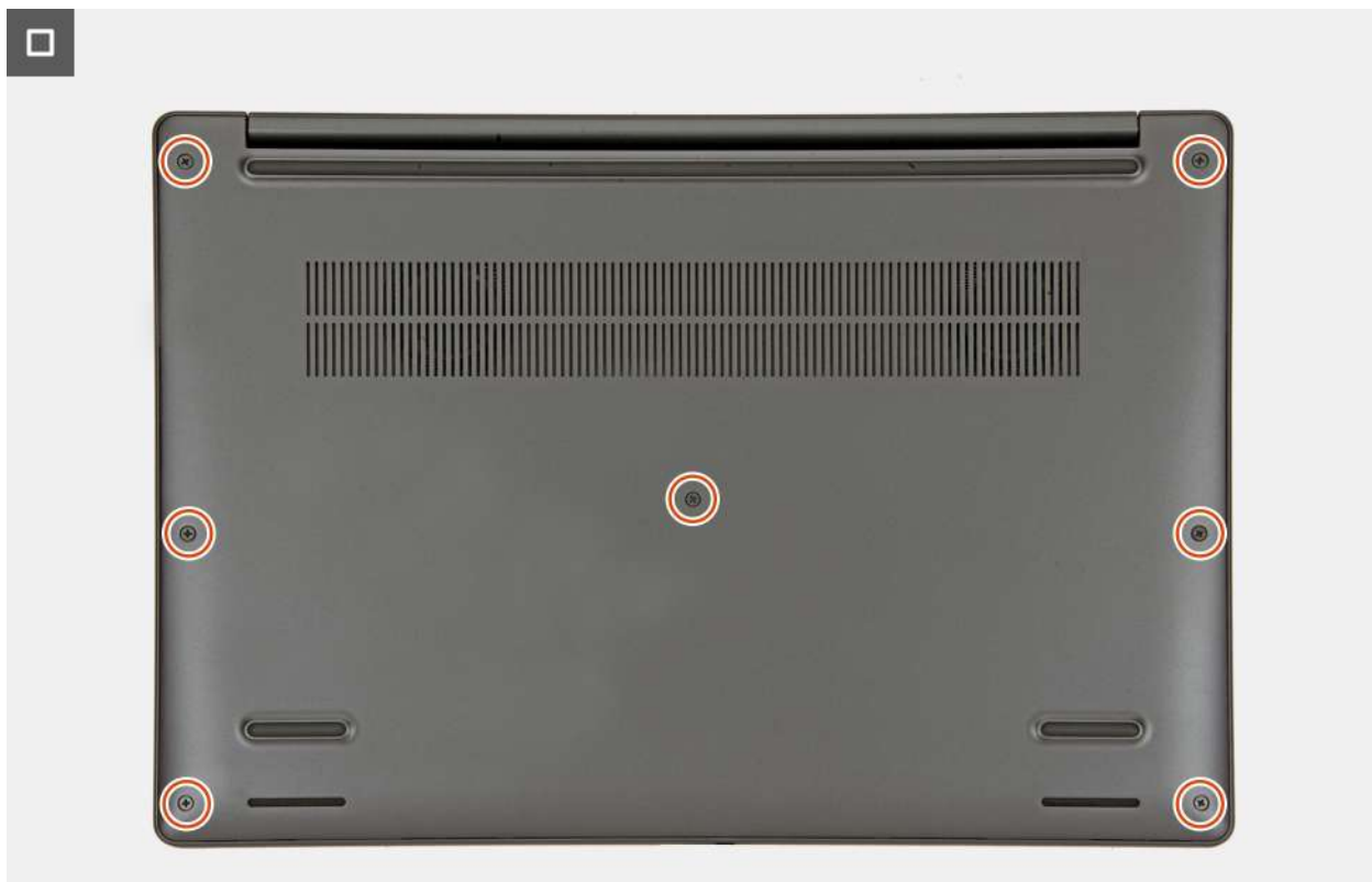
Rysunek 19. Tighten the captive screws
