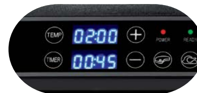
Timer and thermostats with temperature regulation in the range 140-230°C
