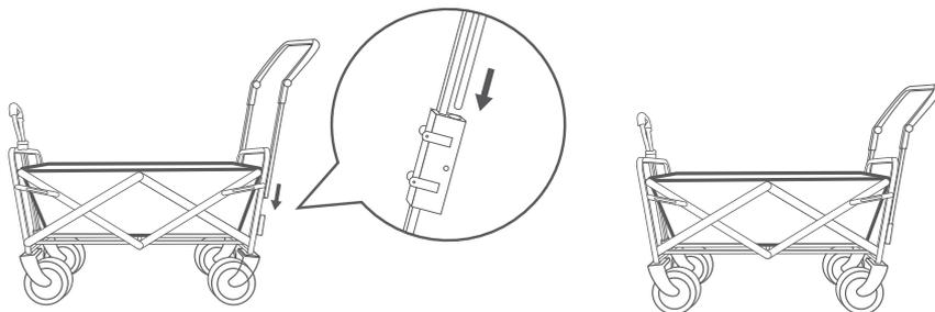
**EN:** Clip the rear push rod fastener into the rear frame (try pushing it in at different angles to get stuck) and fix it with screws. Insert the rear push rod into the fastener, the buckle pops out, and the installation is completed
