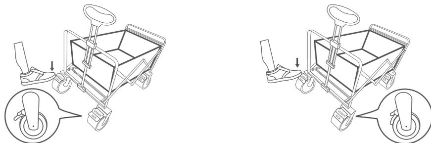
EN: NOTE: FOOT PRESS THE LOCK TO BRAKE AND FOOT PRESS TO UNLOCK TO OPEN
