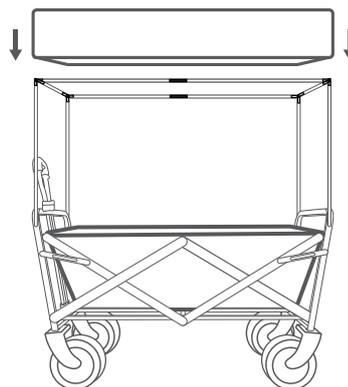
**EN:** Install the four ceiling brackets on the four corners of the vehicle body, fix them with screws, and insert the ceiling into the brackets separately.
