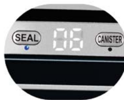
Electronic control panel with LED indicators
