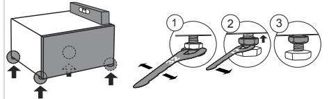
Level the pedestal drawer in longitudinal and traverse direction by rotating the adjustable feet (using a spanner no.32). The feet allow levelling by +/- 1 cm.
