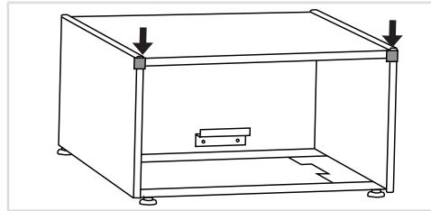
Before the first use, it is necessary to remove all transport protection. The transport elements are intended to protect the pedestal drawer during transport and must be removed before start-up.
