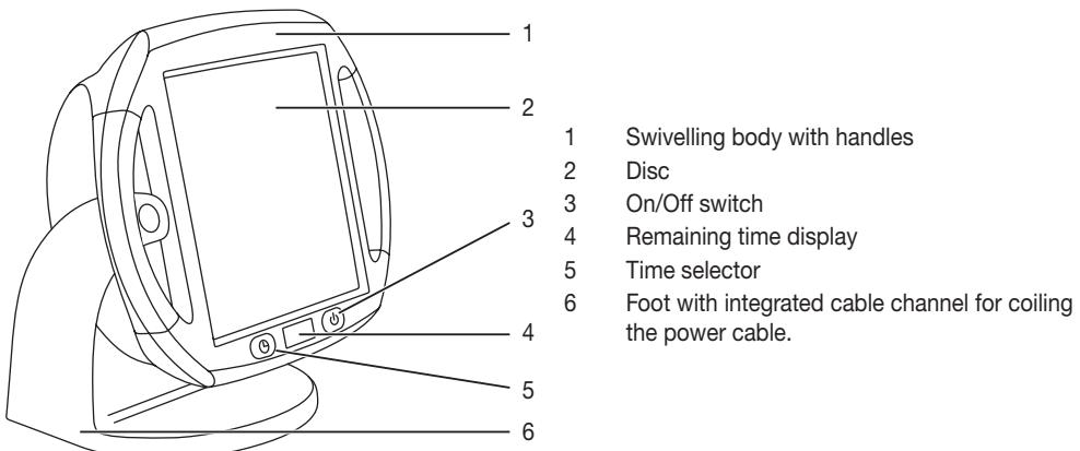
Infrared radiant heater with adjustable timer (1 to 15 minutes) and swivelling body (0 to 50 degrees).
