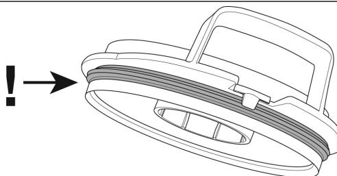
• First, pull the lid over the flange on the mixing bowl, and then push it firmly down on the handle side until the lid locks into place.
