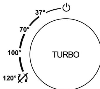
**37 °:** The food is heated to 37 °C and stirred at 200 rpm.
