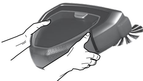
**Always carry the robot with two hands keeping the front up. Manual moving of the robot:**
