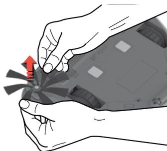
**Pull the Side brush to remove it.** Clean the Side brush. Reattach the Side brush in the socket. Side brush can be changed. (Ref: **ERK2 / EBSB2**)
