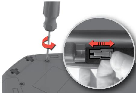
**1. The battery compartments are located on the bottom side of the robot.** Use a screwdriver (PH2) to unscrew the battery compartment lids. Replace the battery packs and refit the battery compartment lids.
