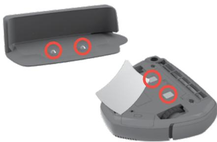
**Use a dry soft cloth to clean regularly the charging connectors** on the charging base and under the machine.
