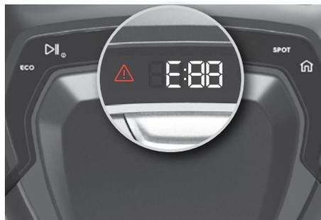
**1. If an error occurs,** the robot stops cleaning. The warning icon will pulse and the digits **"E:" followed by an error code,** is shown on the display. The speaker will also describe the error. After an error has occurred, press any button to play the audio message again.
