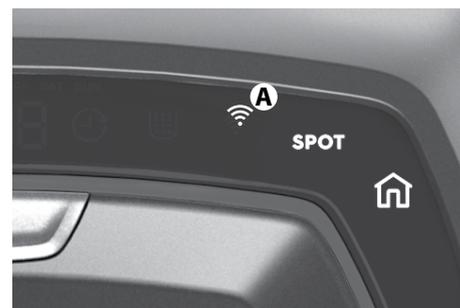
3. When the setup is completed, turn the robot back to its normal position. The WiFi symbol (A) will be lit up to indicate that the robot is connected to your home network. **Note:** it could take a few moments for the robot clock to automatically synchronise with your mobile device.
