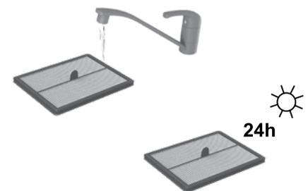
**3. Rinse the filter with cold water.** Tap the filter frame to remove water. Let dry for 24 hours before placing it back in the machine.
