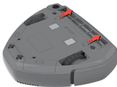
**1. Press the two latches and slide the lid forward to remove the brush roll lid.**
