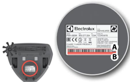
2. During the process the App will ask you to turn the robot upside down to activate the WiFi module and scan the serial number bar code (A) or enter it manually (B).
