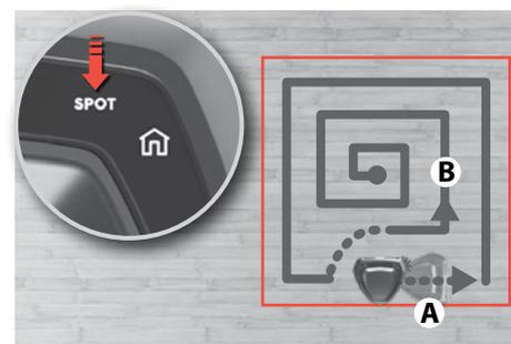
**SPOT cleaning (small area, ~1 m<sup>2</sup>):** Place the robot facing the spot and press the SPOT button. The robot will clean the area twice.
