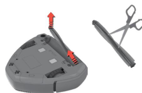
**2. Pull out the Brush roll and clean the brush and bearings.** Remove entangled threads by snipping them away with scissors. Refit in reverse order. Brush roll can be replaced. (Ref: **ERK2**)
