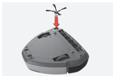
**2. Use the magnetic function to attach the side brush in the socket located on the bottom side of the robot.**
