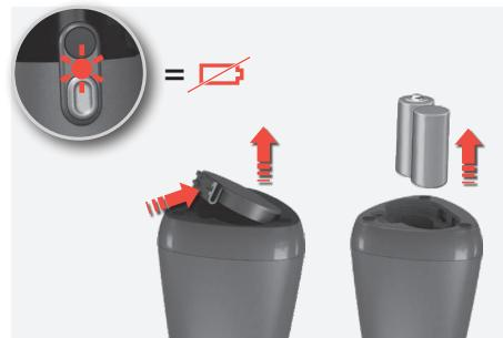
**5. Changing the batteries:** The red pulsing led indicates that the batteries need to be changed. The battery compartment is located on the bottom side of the virtual barrier. Press the latch inwards and remove the lid. Replace the two batteries and refit the battery compartment lid.
