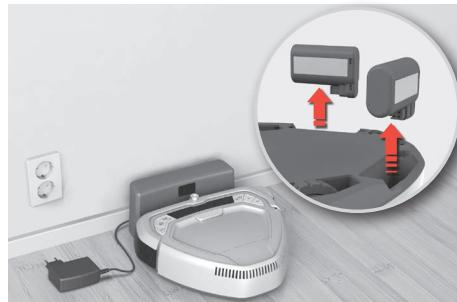
**3. Storage (not plugged):** In case the robot is stored without being charged, remove the batteries and store them separately. (Charge batteries before removing them). *To remove the batteries see instruction "Changing/removing the batteries" on page 32.*
