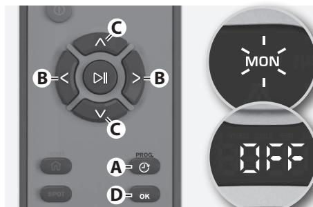
**5. Change "Hour":** press  $\wedge$  or  $\vee$  button (C) until the desired hour flashes. Press "OK" (D) to confirm.
