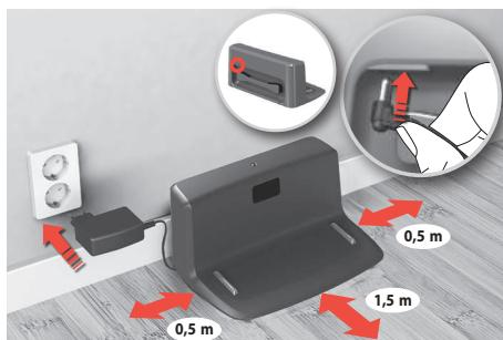
**1. Place the Charging base** on the floor against the wall. Plug the adaptor to the power jack on the back of the base. Connect the Power cord plug to the main socket. Wind up excessive cord on the back of the base. Make sure there is an empty area of 0.5 m on the sides and 1.5 m in front of the Charging base.
