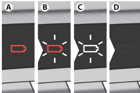
**1. Red battery (A)** indicates that the device needs to get charged.
