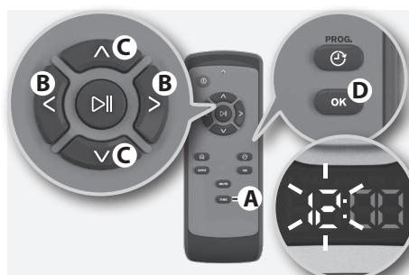
**3. Change "Hour":** press  $\wedge$  or  $\vee$  button (C) until the correct hour flashes. Confirm by pressing "OK" (D).
