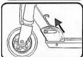
4. Pull the lever upwards.
