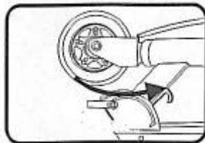
1. Unlock the locking mechanism.
