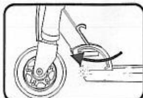
3. Open the locking mechanism.
